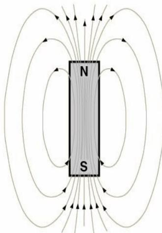
This is a representation of a bar magnet, around and through which are magnetic lines of force. If you lay a piece of paper over the top and sprinkle iron filings on it they will line up with the lines of force, and you can plainly see their shape, orientation, and how many of them there are.
